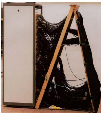
**Figure 1a - The Problem:** Current measuring systems require large numbers of interconnecting cables resulting in added cost, weight, complexity, and lower reliability and performance
