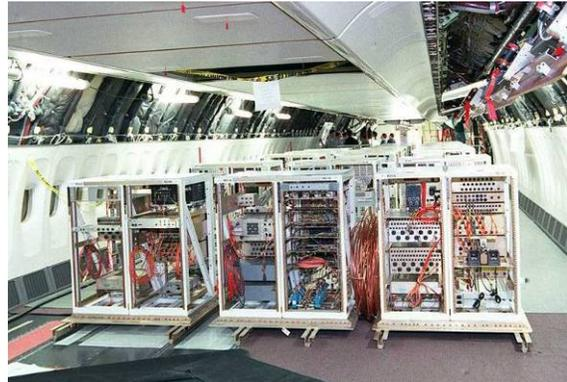
**Figure 2. Flight Aircraft Testing. Instrumentation racks inside Boeing 777 airplane during flight test**
