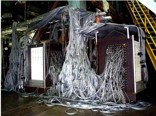
**Figure 1. Ground Aircraft Testing. Bundle of cables covers a jet fighter under structural testing**
